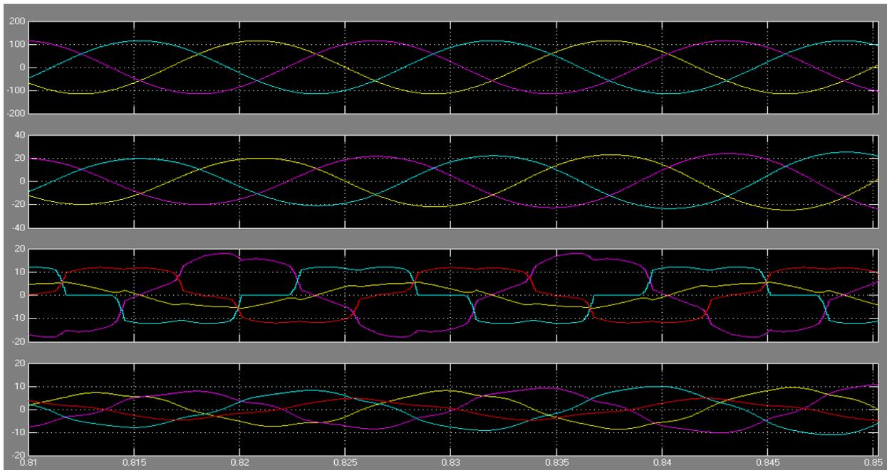
Fig. Simulation results: (a) Grid voltages, (b) Grid Currents (c) Unbalanced load currents, (d) Inverter Currents
