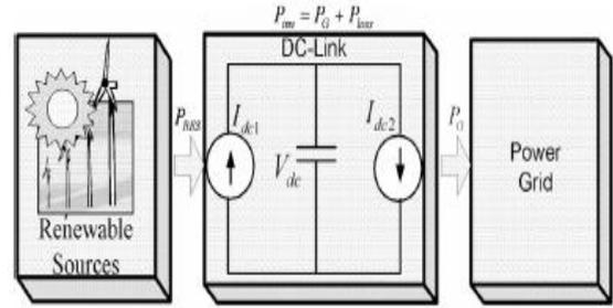
Fig. 2.DC-Link equivalent diagram.
